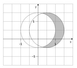
(a) Explain how we can use these two circles and Constructive Solid Geometry (CSG) to create the image of a waxing moon as illustrated by the gray area in the image above.
