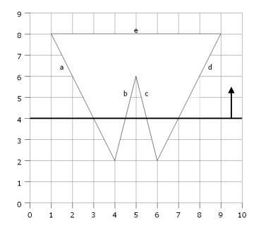
For the scanline approach, we use the two data structures Edge Table (ET) and Active Edge Table (AET).
