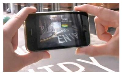
The image on the left shows a handheld AR system implemented on a state-of-theart smartphone, where information that is related to the direction where the phone is pointing at is superimposed onto the live video stream of the phone's away-facing camera.
