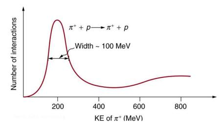
Figure 5: The probability of the interaction between a  $\pi^+$  and a proton as a function of the incident kinetic  $\pi^+$  energy.
