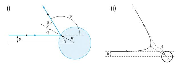
Figure 1: i) Diagram should show scattering at approximately correct angle and with angle of incidence approximately equal to angle of reflection. b and  $\theta$  must be indicated and defined as scattering parameter and scattering angle respectively.  $\beta$  and R are not required. ii) Path should have smooth curve resembling hyperbola at approximately correct angle. b and  $\theta$  must be marked.  $r_C$  and R are not required.
